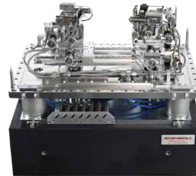
■ Horizontally Dispersing Monochromator in Laue-Laue configuration with fixed exit Double Laue bent crystal (Double bounce) (~ 22.7 ÷ 141.7 keV) European Synchrotron Radiation Facility ESRF- Grenoble (France)
